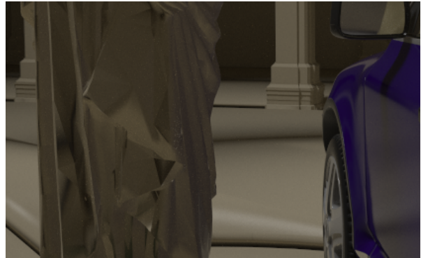
Figure 21: Renaissance scene with floor decimation. Notice the shadowing error that occurs behind the statue as a result of trying to decimate objects with too few polygons. Objects like this floor were manually excluded from decimation to prevent this.
