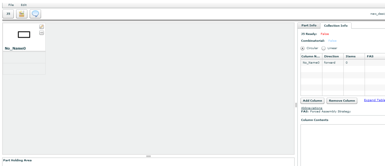
Figure S2: Screenshot of Device Editor when using the program. Users can add columns by clicking on the “Add Column” button on the right pane which allows for additional DNA fragments to be added for final assembly. Sequences can be copied into Device Editor by right clicking under the column in the grey boxes and clicking either “Map from Clipboard” or “Map from File.” Assembly rules like embed sequence in forward/reverse primer, direct synthesis, or digest can be found in Forced Assembly Strategies. Once all pieces and assembly strategies are met, users can mock assemble the pieces by clicking on the j5 button on the tip left of the page (12).
