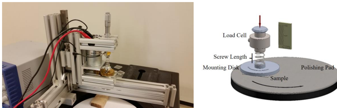
Figure 10. Second generation force-measuring device (left). Schematic depicting the polishing process (right). While the polishing pad (light gray disk) is spinning counterclockwise, a motor rotates the mounted sample (light blue disk) clockwise to ensure the Au-plated surface is evenly polished. Compressing the load cell converts the mechanical force into a digital voltage reading that is directly proportional to the applied force. Reproduced with permission from Harry Hu.
