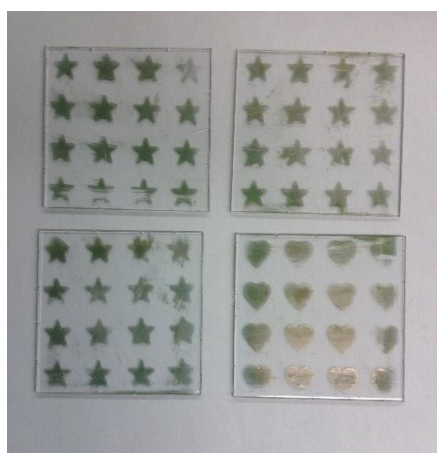
Figure 28. 140.7 \pm 34.8 Å thick Au thin films patterned by post-deposition \text{CHCl}_3 vapor exposure.
