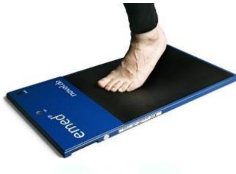
Figure 8. The Pressure mat used for barefoot testing, which was embedded in the laboratory floor. (42)
