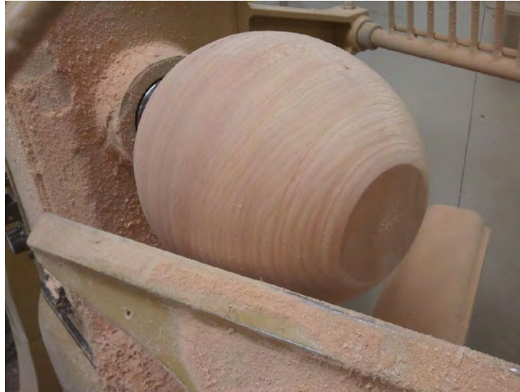
Figure 22. Starting on the lathe Once the pieces were dry, I put the cylindrical shape onto the lathe and began shaping the form with a hand
