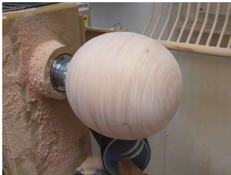
Figure 23. Still turning Turning the shape on the lathe took a couple of hours of shaping and reshaping
