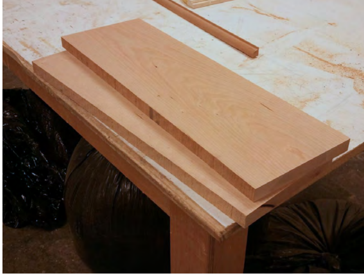
Figure 19. Joining and planing I joined, planed, and cut the wood into large pieces to work with
