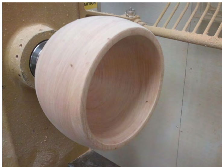
Figure 24. Turning the inside Once the exterior shape was finished, I cut the top part of the sphere off for the lid, and I hollowed the interior using a similar shaping method
