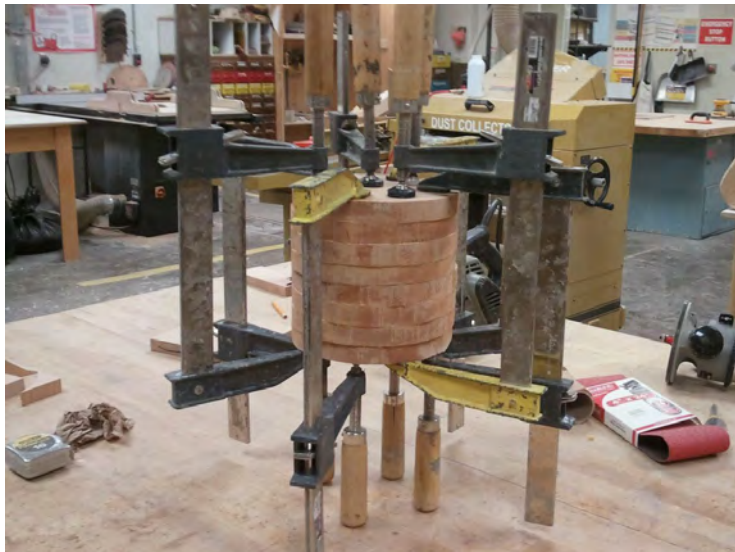
Figure 21. Gluing up After cutting all of the pieces into circles, I glued them on top of each other, roughly matching the wood grain, then clamped
