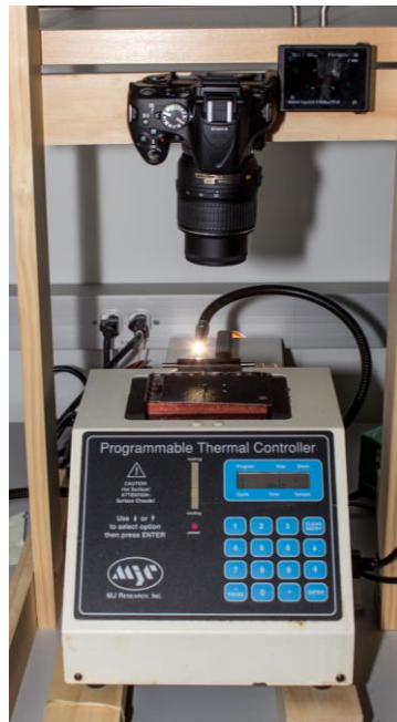
Figure 6. Experimental set up for the cold behavioral assays. Larvae were placed on a black metal plate and the plate was then placed on top of the chilled thermocycler block. Larval behavioral responses were video-recorded with the Nikon Camera.
