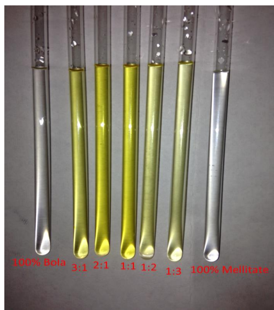
Figure 11: Different ratios of (M-1,1) 2 -12 to mellitate in DMSO-d 6 /D 2 O (7/3). From left to right the [bolaamphiphile]:[mellitate] decreases, while [bolaamphiphile] + [mellitate] is kept constant at 4.2mM.
