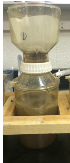
Figure 8. Sample is placed on filter paper and vacuumed to remove high density LST, which can be seen collecting in the bottom of the container.
