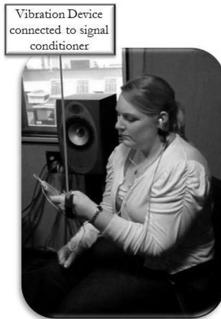
Figure 4. Vibro-tactile Feedback System. Subject using the Vibro-tactile Feedback system; device attached to the back of the same hand used for adjusting the iPod
