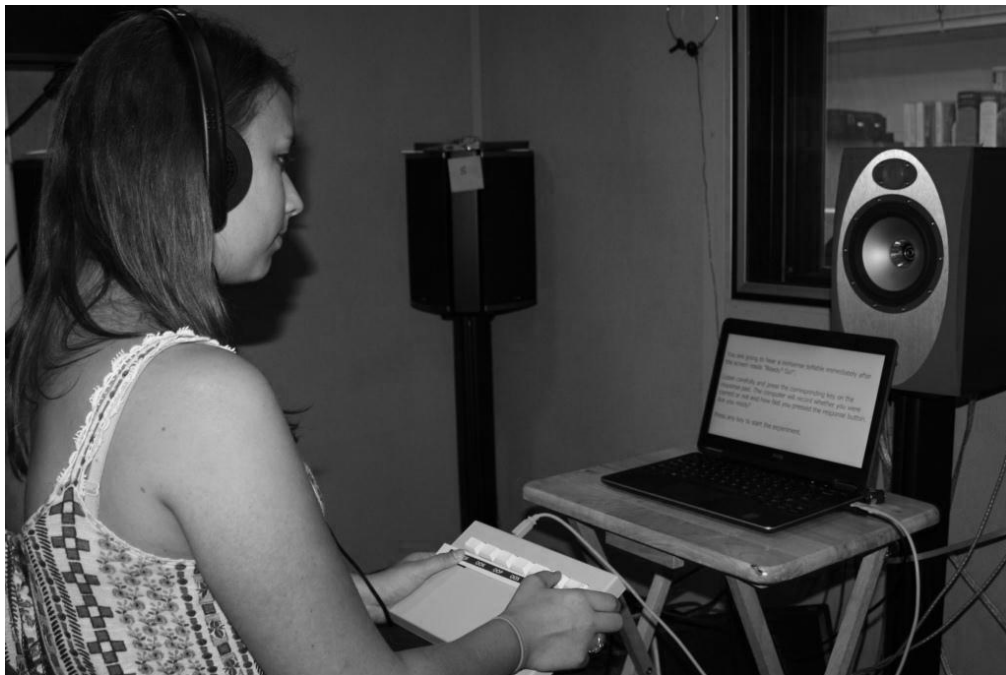
Figure 2. Equipment set up; left panel- real ear measurements were taken with the iPod headphones; right – the reaction time task with the laptop and Cedrus response pad.
