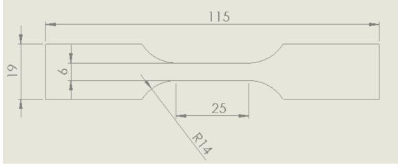
Figure 31: Drawing of the IV specimen (All dimensions in mm).
