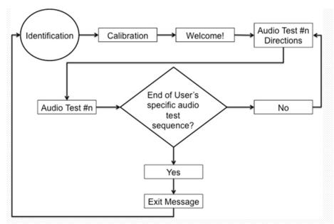
Figure 3. Conceptual process for taking of audio test.
