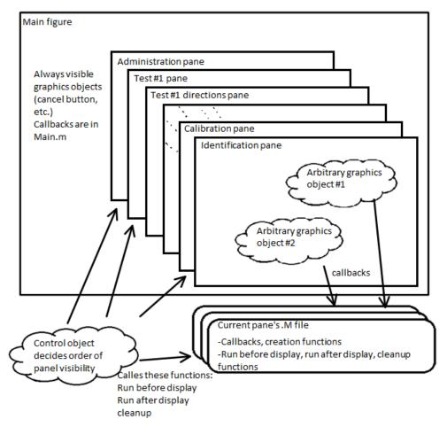
*Figure 7.* Framework used in the GUI. Any number of uipanels can be added to allow addition of another audio test, more instructions, etc.
