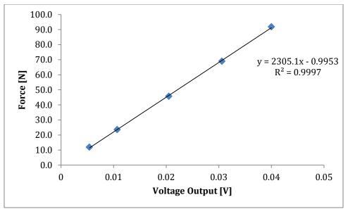
Figure 26: The Calibration Equation for the Load Cell
