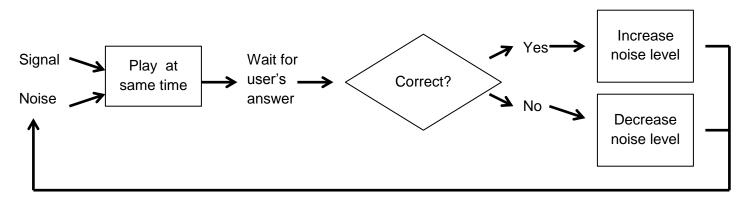
Figure 9: Design of Speech in Noise Hearing Test (excludes Training Loop)
