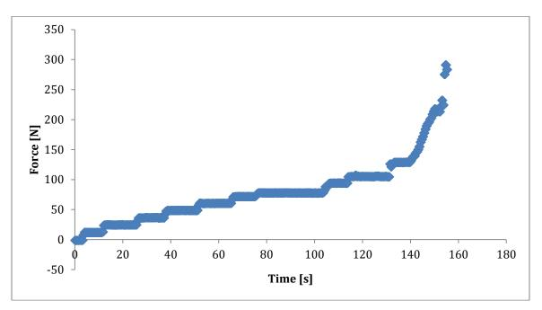
the calibration equation was used to convert the voltage output to a force. Figure 23 is a graph of the force applied to the load cell.
