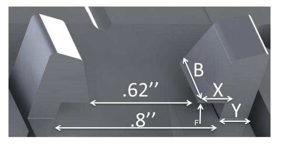
Figure 37: Dimensions of Speaker Hooks
