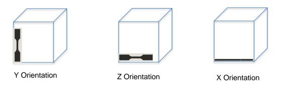
Figure 32: Orientation of Specimens
