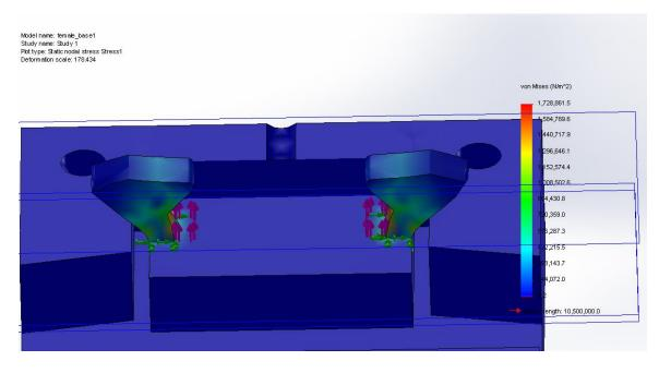
Figure 38: Static Simulation in Solidworks
