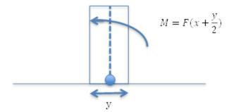
Figure 20: re-simplified model of clip attachments
