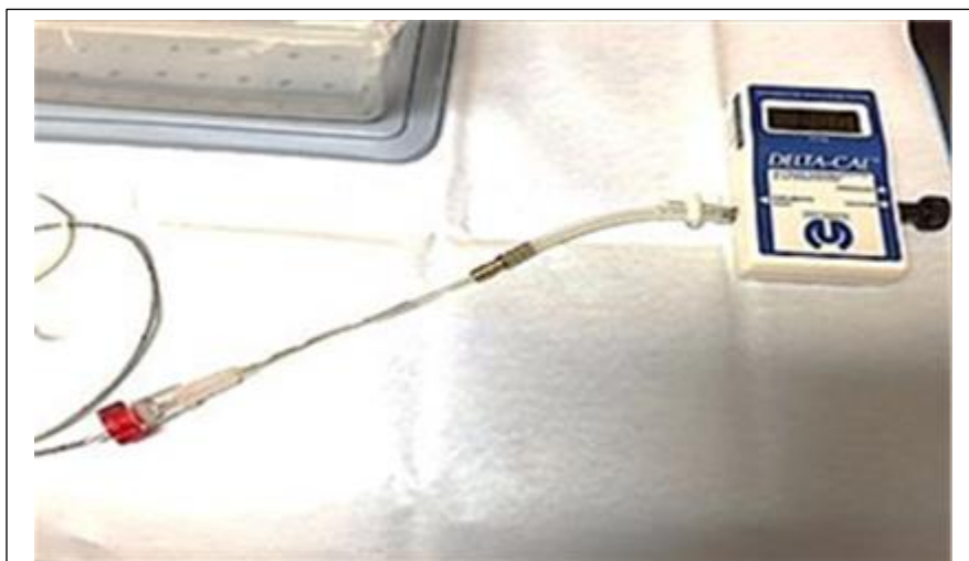
Figure 2. Manometer calibration. Catheter is inserted into pressure chamber of the Delta-Cal digital pressure calibrator.
