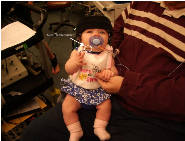
Figure 6. Infant participant wearing NIRS probe headband and “suck” accelerometer (circled in white). “Swallow” accelerometer not visible in picture.
