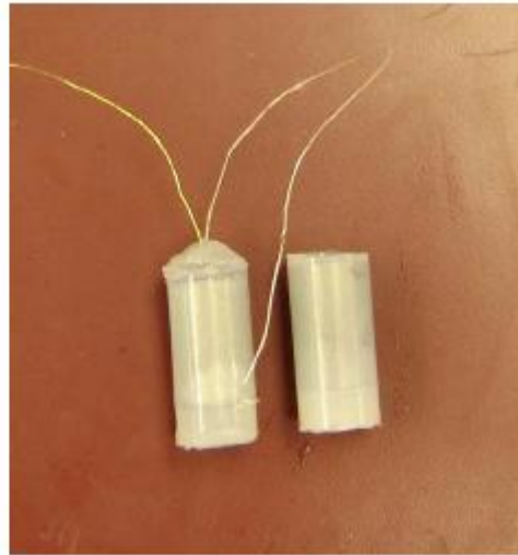
Figure 4: Schematic structure and picture of the fabricated CO 2 sensor designed by Ningliu.
