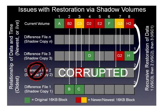
Figure 8: Shadow Volume Restoration Issues caused by Corrupt/Missing Shadow Copy #2
