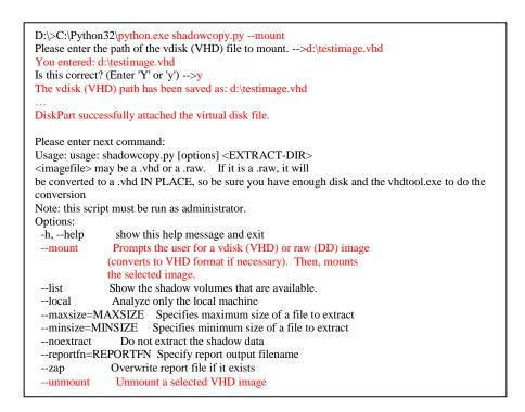
Figure 22: Execution of shadowcopy.py to select and attach a virtual disk image (VHD) file
