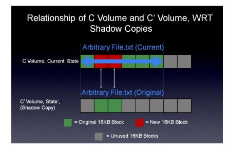
Figure 4: Relationship of Structures and Data on live (C) Volume and VSC (C') Volume
