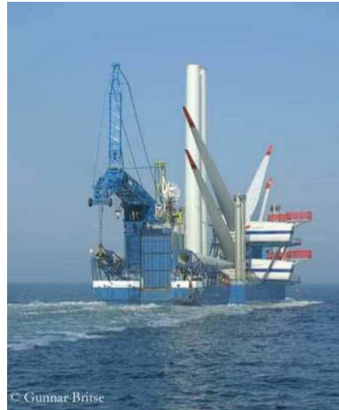
Figure 16: The crane vessel “Ocean Hanne” which was used for the transportation and installation of the wind turbines. 95
