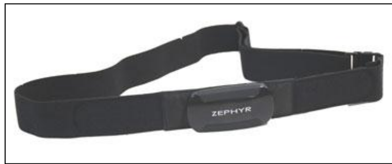
Figure 22. The HxM™ BT module (device with Zepher written on it) and the Zephyr Bioharness for monitoring a person's heart rate, speed, and distance.
