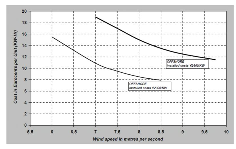
Chart E3: Cost of wind energy for offshore wind farms constructed in 2007 shown as cost/kWh plotted against wind speed, indicating that to be cost effective the offshore wind must be in an area with high wind speeds[A5]
