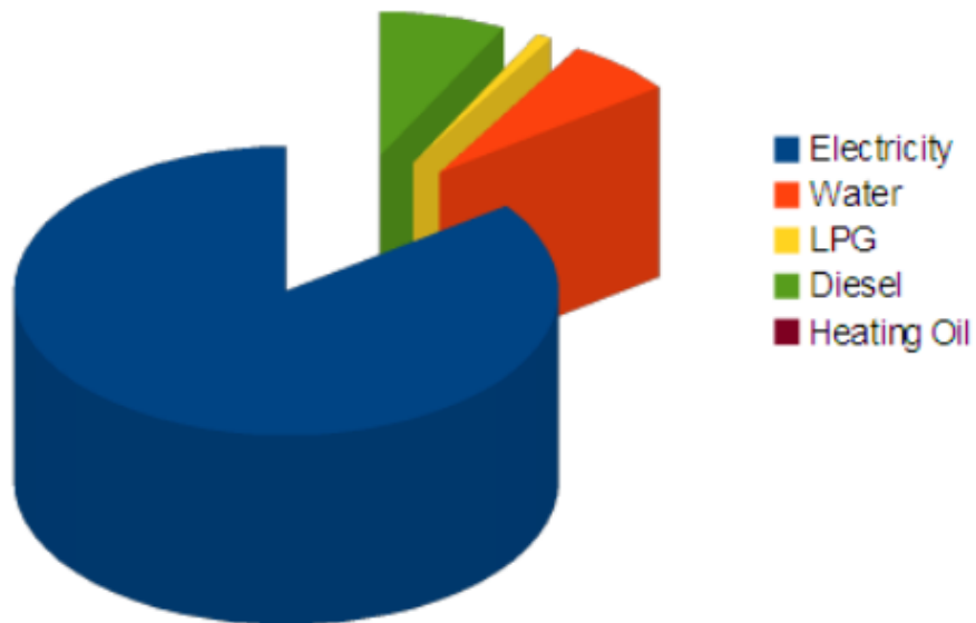
Distribution of 2386.2 tonnes of CO2 per annum amongst different sources of energy for Coastline Hotel
