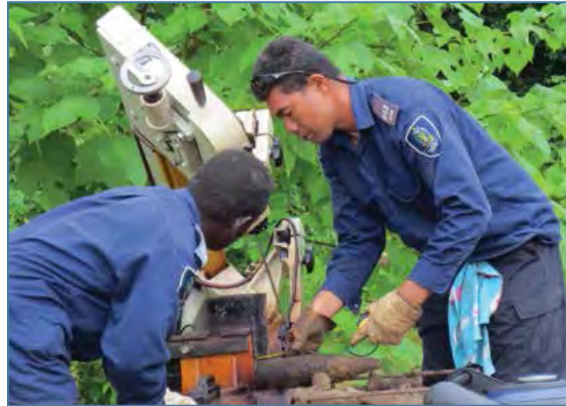
Members of the Royal Solomon Islands Police Force are trained in explosive ordnance disposal (EOD) by Golden West Humanitarian Foundation. Here, two of the EOD team members cut a World War II-era projectile at the team's EOD facility at Hell's Point on Guadalcanal.
