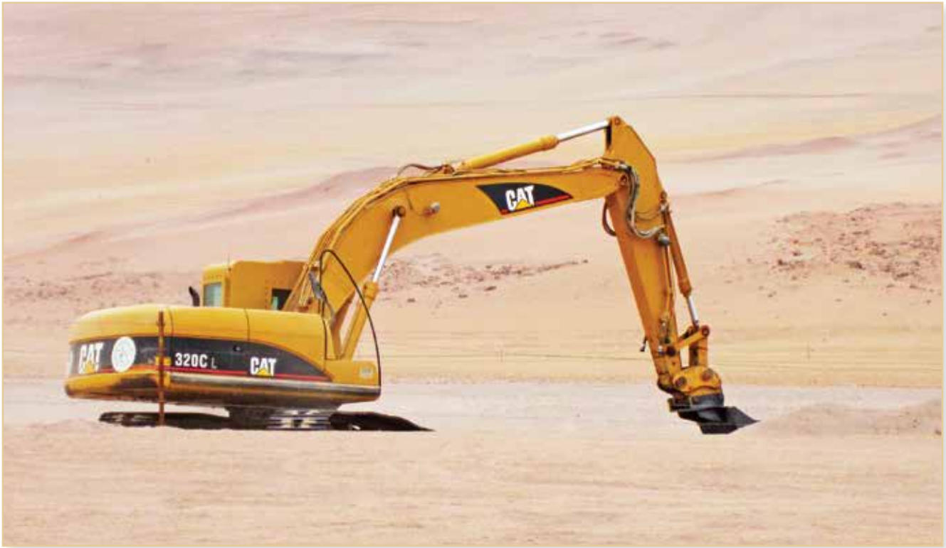
The Multi-Tooled Excavator with an armor protected cab works deep in a dry creek bed to clear anti-tank and anti-personnel mines. Photo courtesy C. Wanner, U.S. Dept. of Defense, Humanitarian Demining Research and Development Program.
