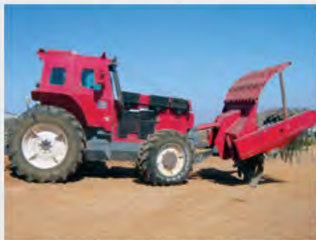
The United States provided this ARMTRAC 100 armored tractor with a flail attachment to the Lebanese Armed Forces to clear persistent landmines in areas where the type of mine threat and the terrain are ideally suited for mechanical clearance. The logo of the U.S. Humanitarian Mine Action Program is visible on the tractor's cab.
