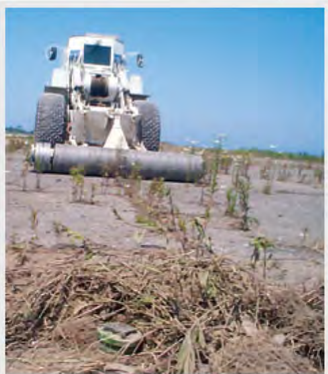
The HALO Trust uses an armored vehicle with a heavy roller attachment to perform "area reduction" in Georgia. A PMN-2 anti-personnel landmine, visible in the foreground, was destroyed less than a minute after this photo was taken.
