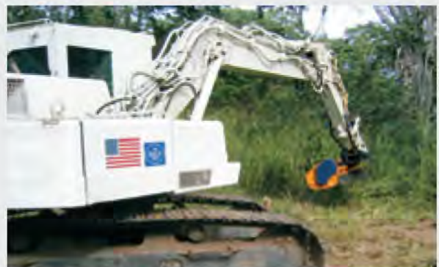
An Atlas Copco tractor with a brush-cutting attachment, provided to The HALO Trust by PM/WRA, clears high grass, brush, and shrubs from a mined area in Mozambique. Next, a deminer can sweep the ground for mines with a metal detector and easily excavate those that are found. When conditions, such as terrain, roads, bridges, and technical support permit, mechanical brush cutters can accomplish in minutes what it takes a manual deminer many hours to do, significantly improving productivity.
