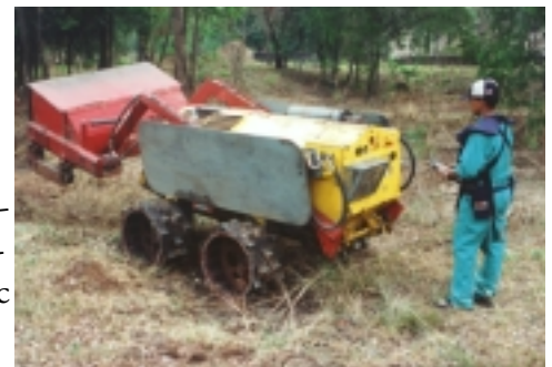
In 2000, the Tempest vegetation clearing machine underwent testing in Thailand.
