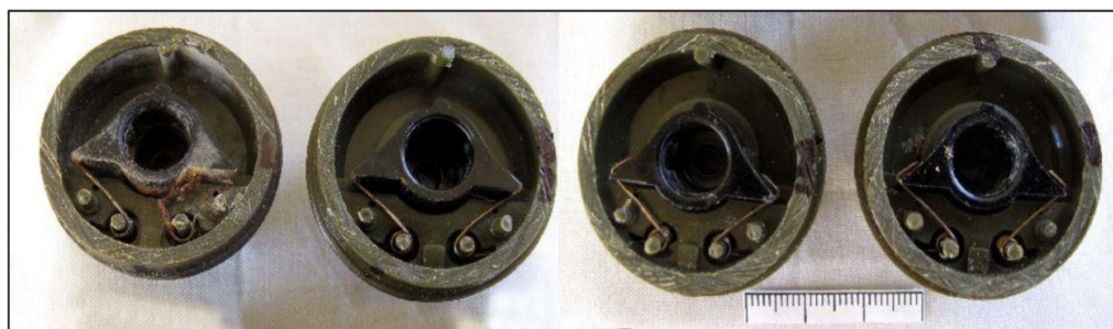
Comparison of the striker wires in position within the fuze housings. Wires in the left hand fuze show substantial corrosion, with one having collapsed completely. Those in the other three fuzes have only superficial rust and retain their functionality.
