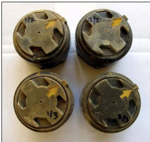
Despite long-term exposure to the sun, the upper surfaces showed very little deterioration
