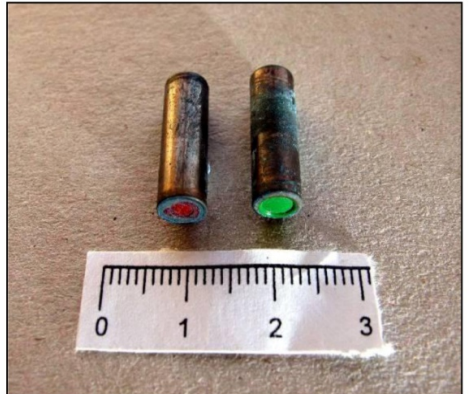
Detonators were in excellent condition, with minimal surface degradation
