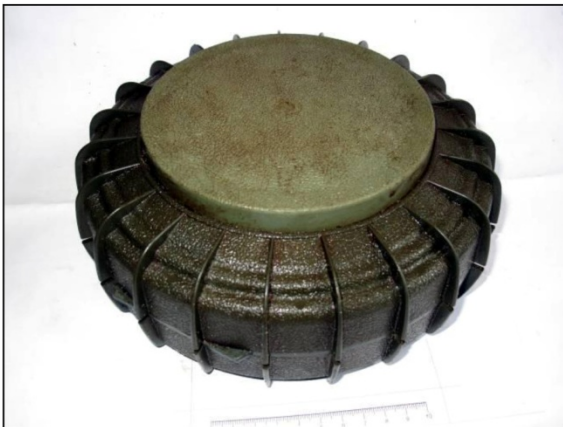
Figure 3: An SB-81 recovered from the Falklands
