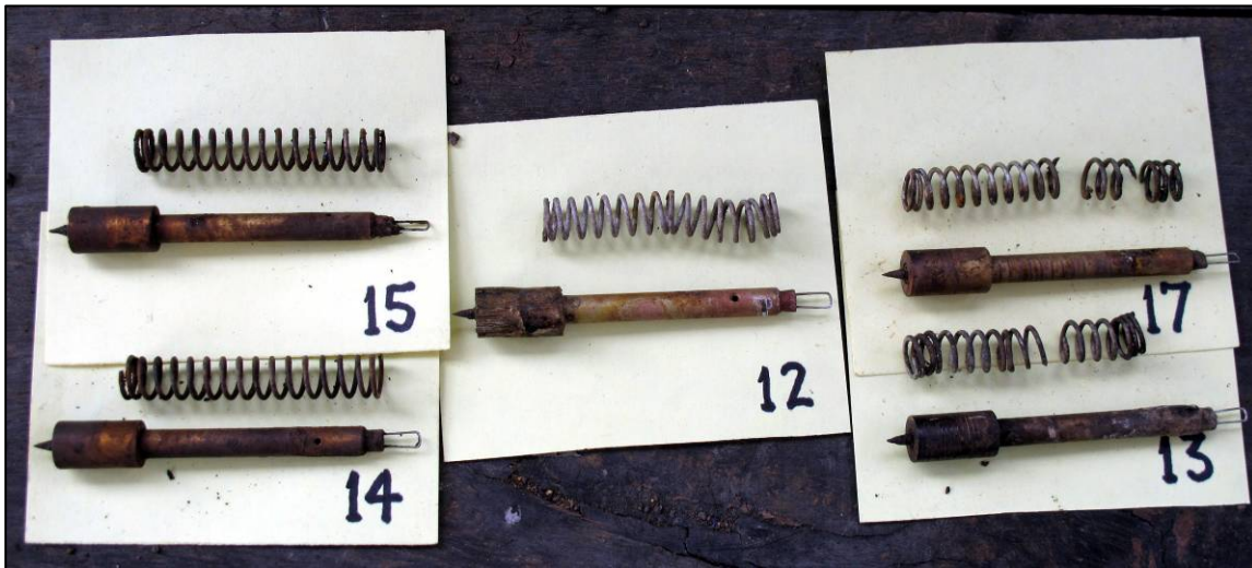
Strikers and springs showed substantial variation in the degree of degradation
