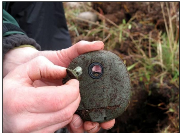
Disarming the SB-33 by unscrewing the detonator assembly from the base of the mine
