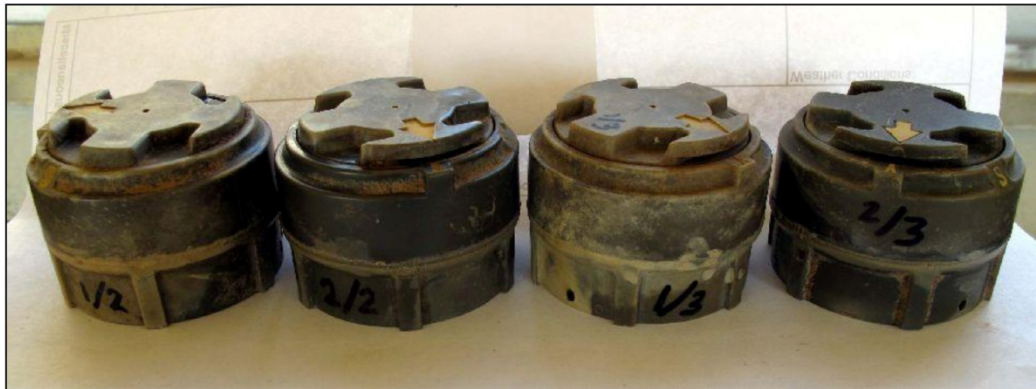
The plastic casings had faded to varying degrees, but were still intact and robust
