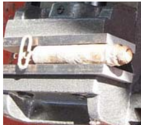
Figure 5. The fuze from a PMD-6, held in place by a bench vice.
