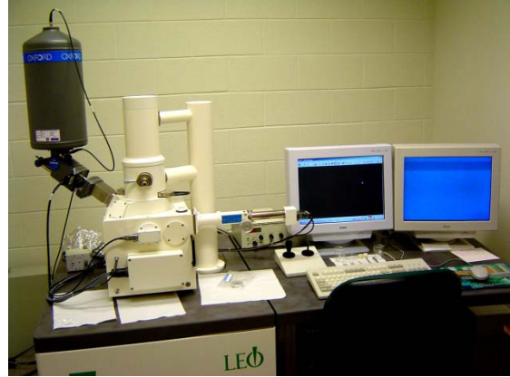
Textures and qualitative compositions of metal parts and materials produced by corrosion are analyzed using the Scanning Electron Microscope at JMU
