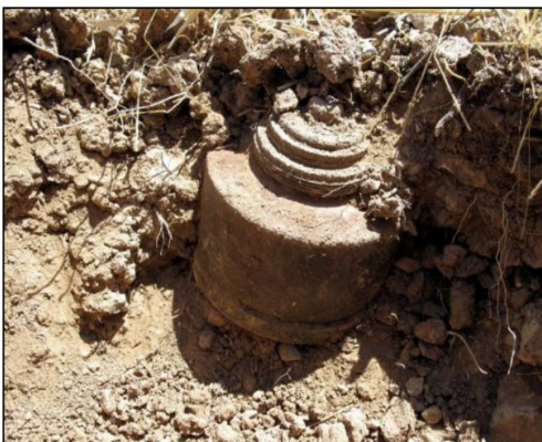
This M35 mine, located well beneath the surface, shows very little distortion
