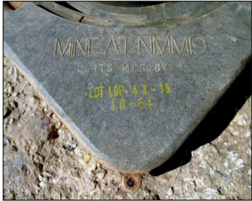
The mine casings, manufactured in 1964, showed no significant signs of deterioration
