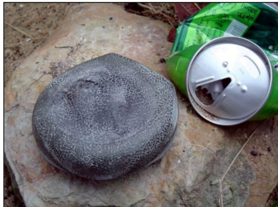
Figure 4: The normal appearance of the SB-33, with a relatively flat pressure plate
