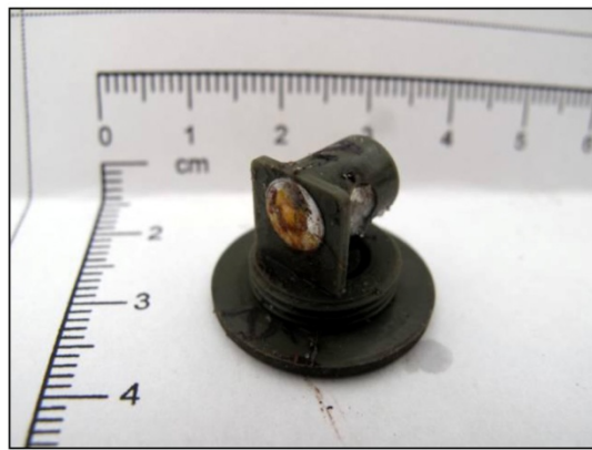
Figure 11: The yellow seal on the stab receptor appears to have been breached
