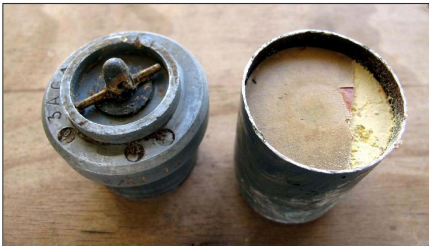
The two fuzes examined were in exceptionally good condition and appeared to be fully functional. The large tetryl booster at the base of the fuze (seen separated on the right of this image) was in perfect condition
