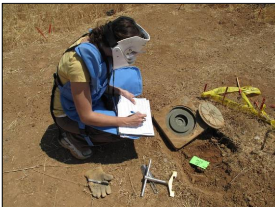
Every step of the process is recorded, along with the coordinates of the mine
