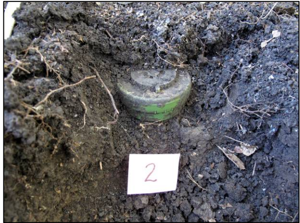
The soil type, burial depth and appearance of the mine are typical of the Type 72s recovered
