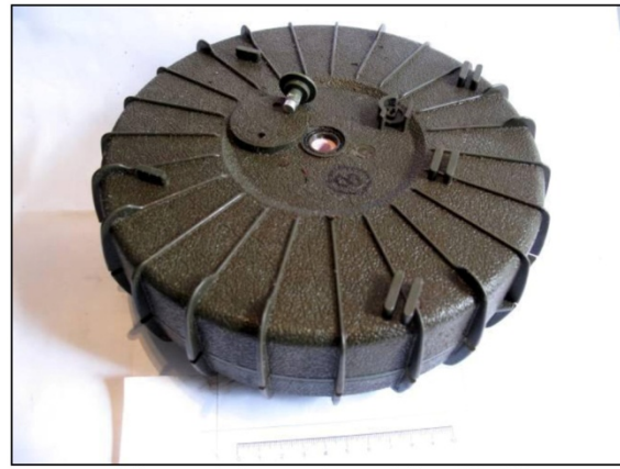
Figure 4: Base view of the SB-81
