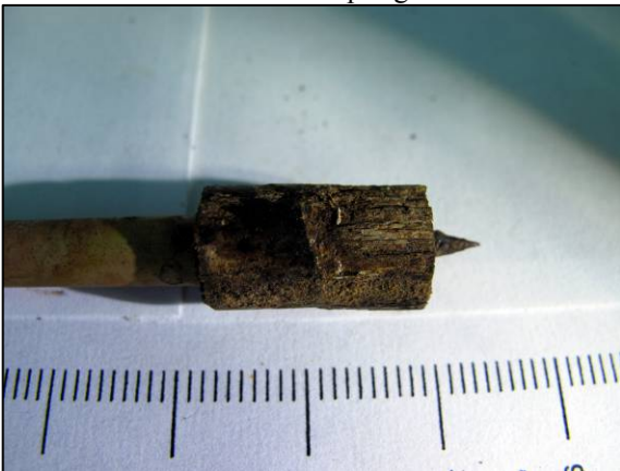
Striker 12 was badly corroded and seized; this would have prevented operation
