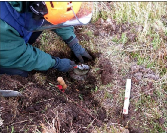
Cut turf was removed in blocks to expose the entire body of the mine
