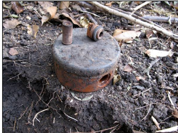
The PMN with detonator removed; in some mines the detonator could not be extracted
