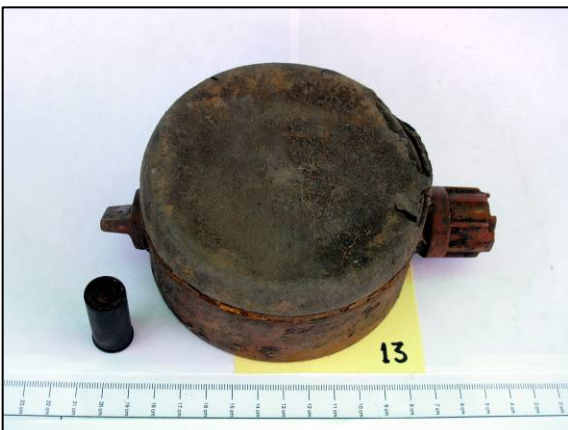
Some of the rubber covers were damaged, allowing water to enter the mine body
