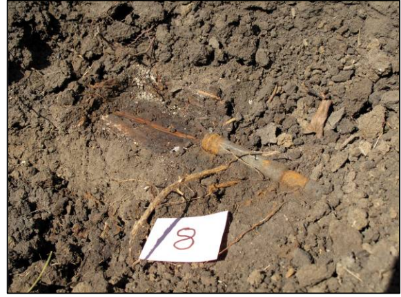
Remnants of the wooden casing are visible once the TNT charge has been removed
