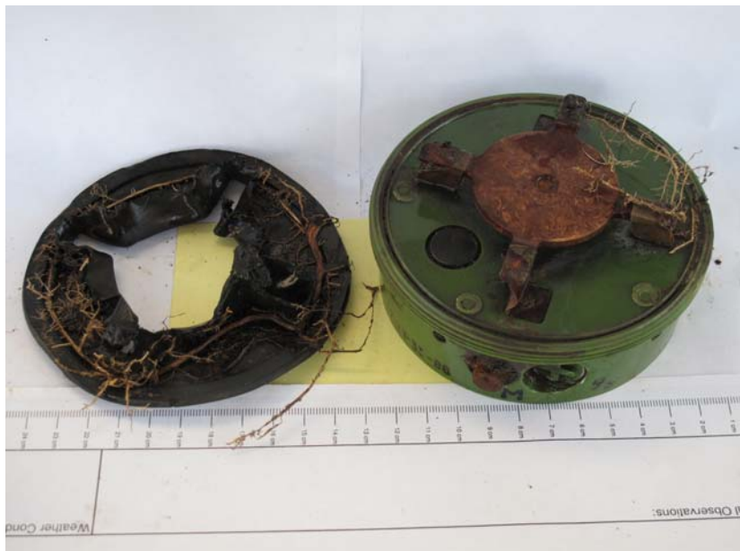
Figure 4. PMN-2 with the top and rubber covering removed, showing root infiltration under the pressure plate.
