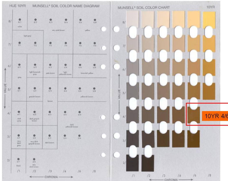
Figure 4. Example of a page from a Munsell color book used to quantify soil color.
