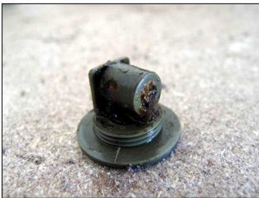
Figure 10: Some detonator capsules did show significant signs of degradation
