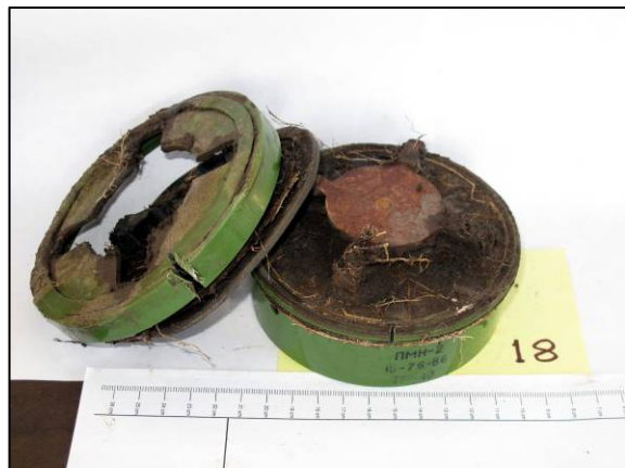
Removal of the securing ring reveals the penetration of soil and roots
