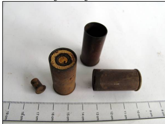
Most detonator capsules were functional, confirmed by explosive testing
