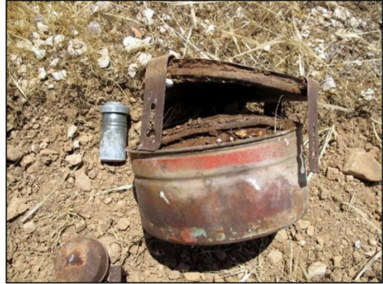
The base of the mine had become detached, with the explosive charge crumbling inside
