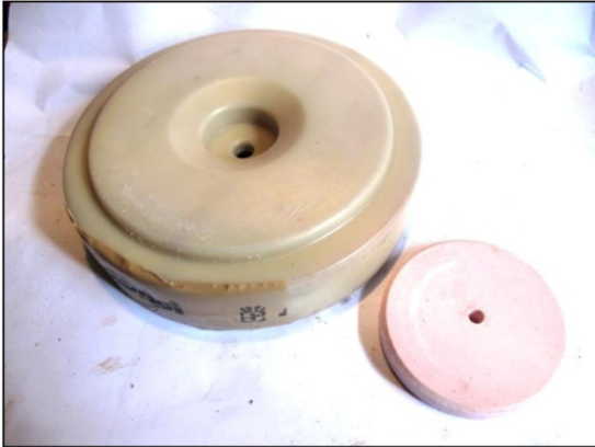
Figure 8: The main charge and booster
