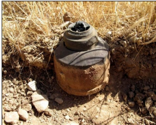
The casing of this mine is distorted, probably from expansion during grass fires
