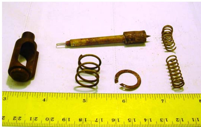
Figure 2. Internal PMN components. The spring pieces to the far right are the striker spring, and the spring to the center holds the cylinder up.
