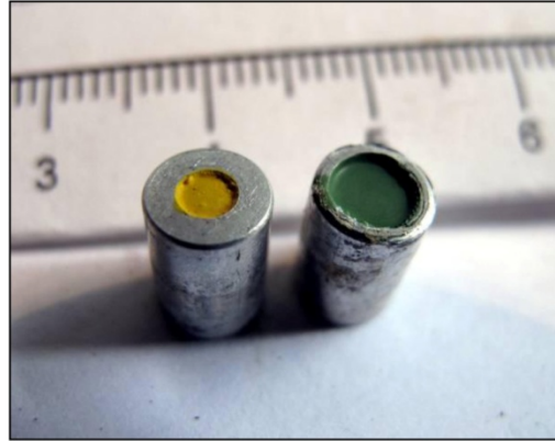
Figure 9: The end seals of these detonator capsules show no signs of deterioration
