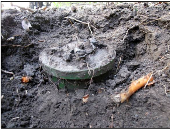
Deterioration of the rubber pressure plate cover
