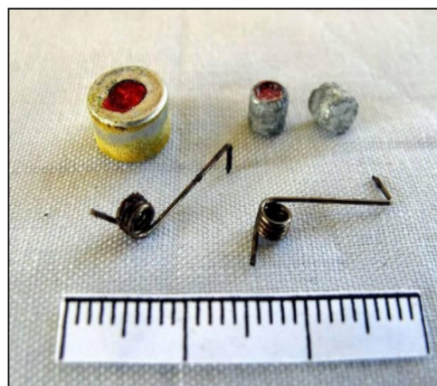
The spring wires in the foreground serve as strikers and firing pins; most were in good condition
