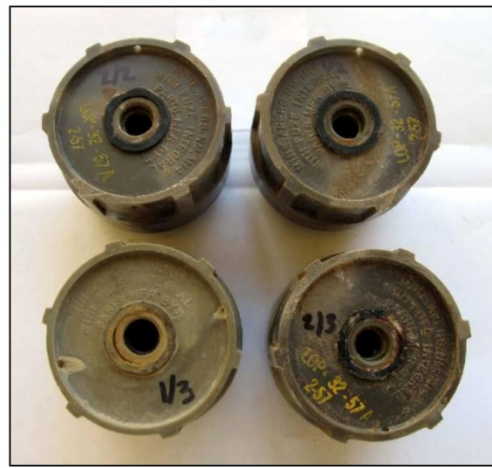
The bases were in good condition, with markings still legible. Rubber seals had hardened
