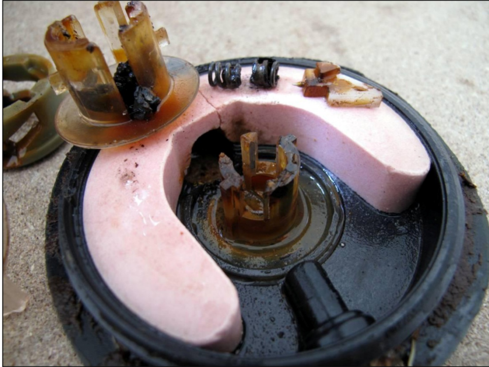
Figure 12: Inside an SB-33 which had been penetrated by water. The most likely cause of failure would be the disintegration of the striker spring, although degradation of the detonator capsule might also prevent the mine from operating. Note that the stainless steel firing pin is virtually unaffected
