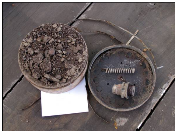
In some cases, soil had almost filled the void beneath the pressure plate
