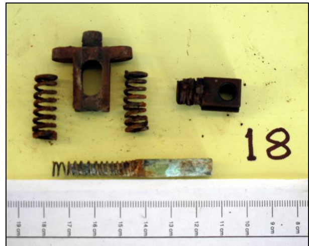
Components of the fuze mechanism, showing that all springs were badly rusted. The plunger (top left) and striker (below) were firmly seized into their channels
