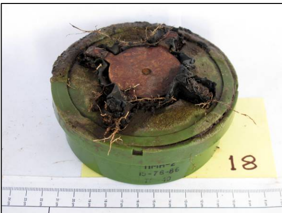
The mine cleaned to show the extent of the rubber and casing degradation
