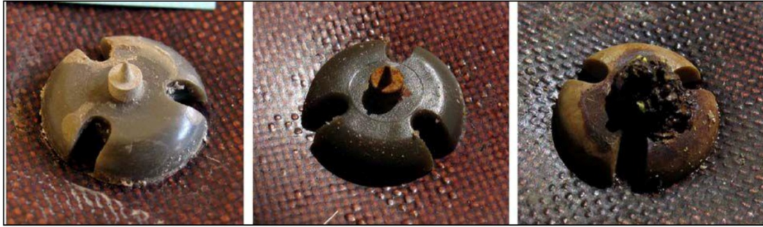
The mild steel firing pins had rusted to varying degrees, but most showed only superficial corrosion
