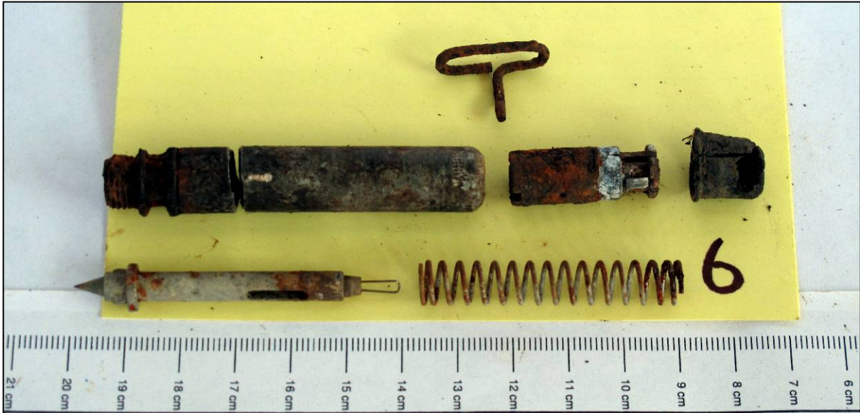
The mechanical components of fuze 6 might have been operational, but it is unlikely that the stab receptor would have functioned
