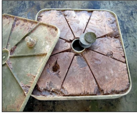
Base plate removed to expose the main charge and booster; both were in excellent condition
