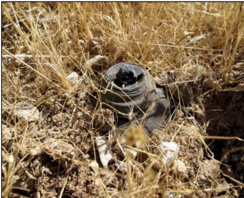
This M35 (No.1) was protruding slightly from the surface, and has a damaged fuze
