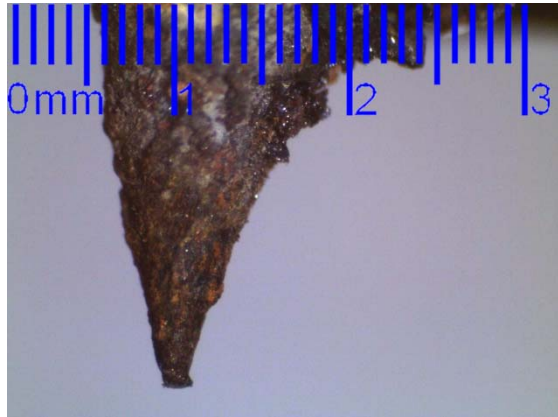
Surface corrosion of metal parts is documented using binocular microscope
