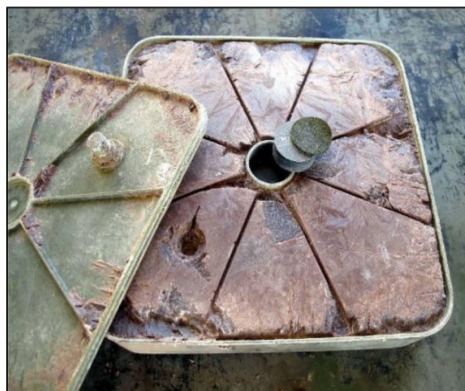
Base plate removed to expose the main charge and booster; both were in excellent condition
