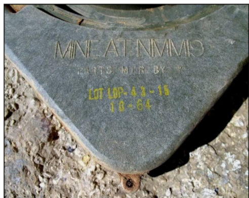
The mine casings, manufactured in 1964, showed no significant signs of deterioration
