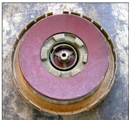
This large Belleville spring raises the operating pressure over 100 kg; it appears to be as new
