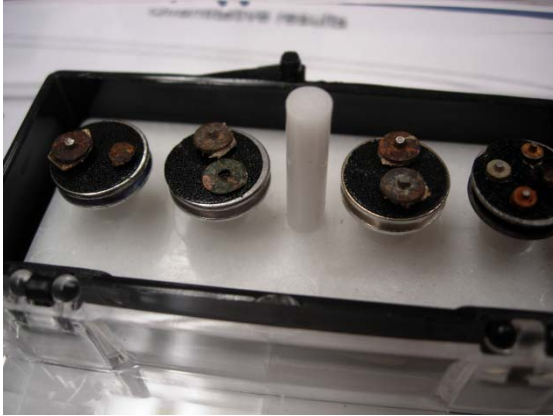
Samples are mounted on carbon-coated Scanning Electron Microscopy mounts
