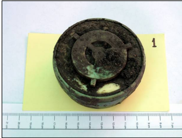
With the rubber cover missing, the Type 72 is penetrated by water and soil
