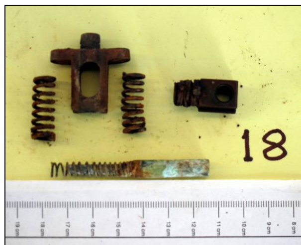
Components of the fuze mechanism, showing that all springs were badly rusted. The plunger (top left) and striker (below) were firmly seized into their channels
