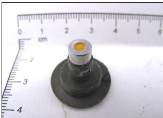
Figure 10: Some detonator capsules showed significant signs of degradation
