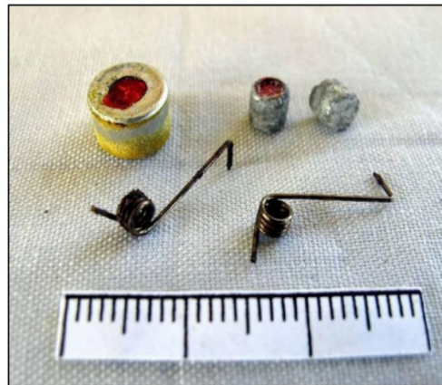
The spring wires in the foreground serve as strikers and firing pins; most were in good condition
