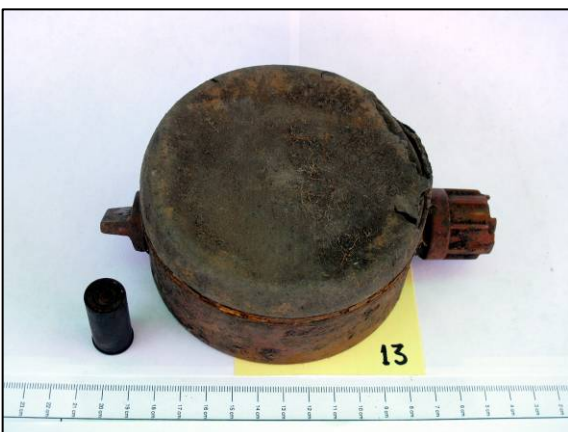
Some of the rubber covers were damaged, allowing water to enter the mine body
