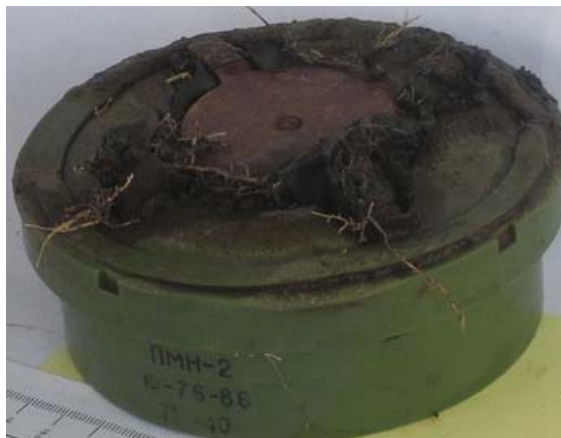
Figure 3. PMN-2, as recovered from the field (after rinsing).
