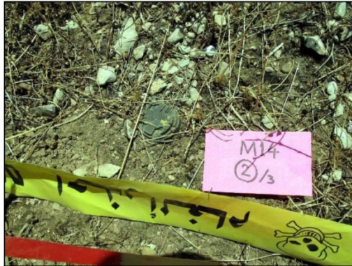
Most of the M14s were flush with the ground level so that the pressure plate was exposed
