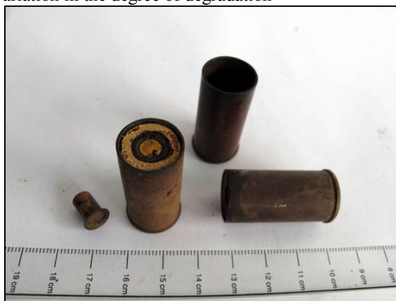
Most detonator capsules were functional, confirmed by explosive testing
