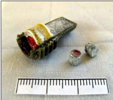
Most detonator and igniter capsules appeared to be functional (scale in mm)
