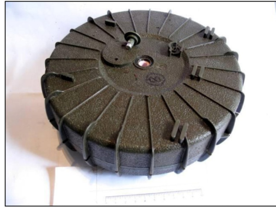
Figure 4: Base view of the SB-81
