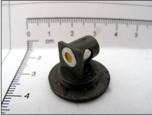
Figure 8: Most detonator assemblies were in very good condition
