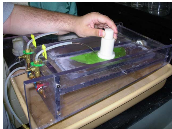
Cut surface is polished with diamond paper to expose cross-section
