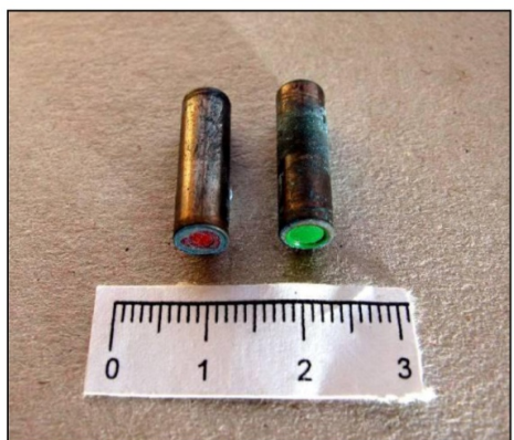
Detonators were in excellent condition, with minimal surface degradation
