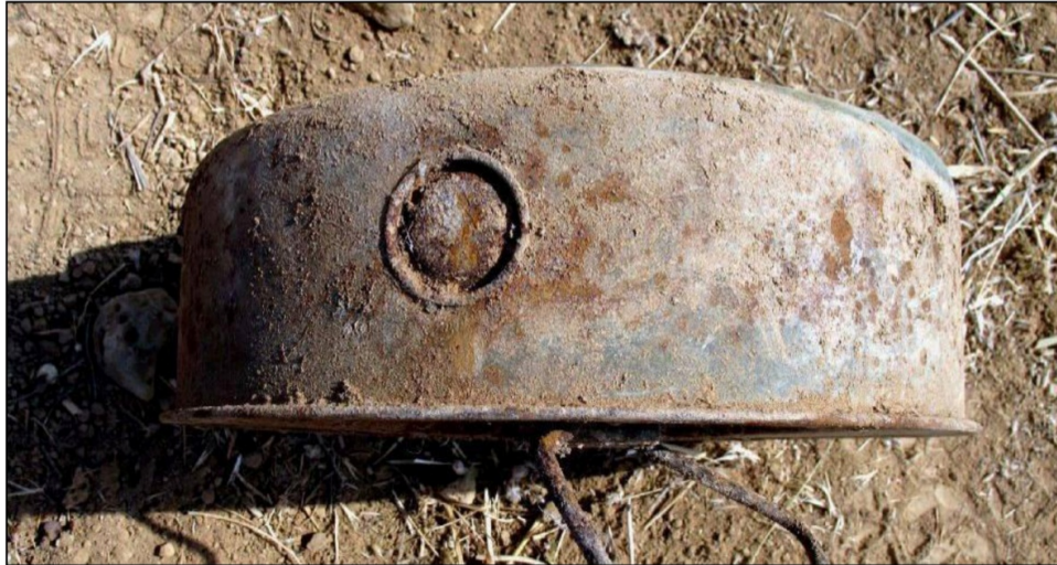
The side of the mine was the area most affected by rust, but neither of the casings was penetrated. The filler plug appeared to be particularly vulnerable
