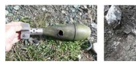
Burned out mortar shell (left) and deflagrated munition (right).
