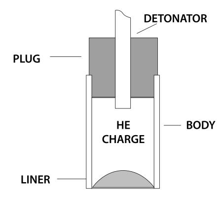
Figure 1. EFP Disruptor components.
