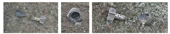
New liner three: in both mortars, the HE burned to deflagration.
