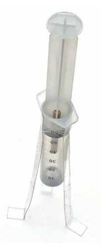
An improvised and low-cost disruptor body with all of the variable control features of those used in our tests.
