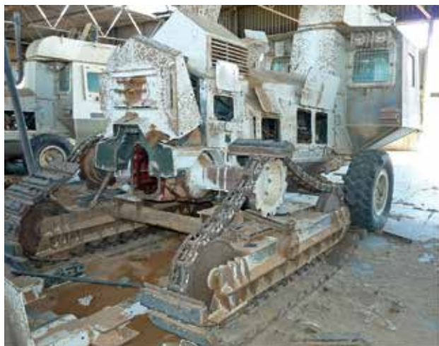
Left, a blast damaged Aardvark flail in Libya and right, blast damaged demining machines in Angola.
