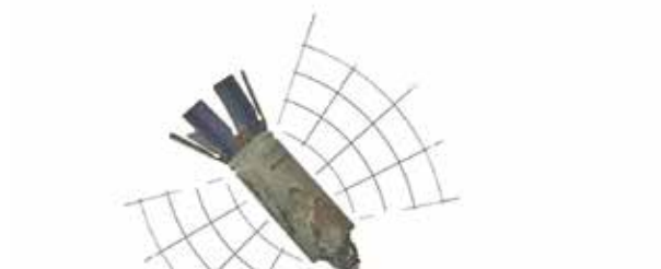
Figure 2. Probable fragmentation dispersion from a 9N210 submunition on a flat hard surface. Fragmentation from such a submunition is dispersed radially with that projected downward scarring on the side from which the submunition came.
