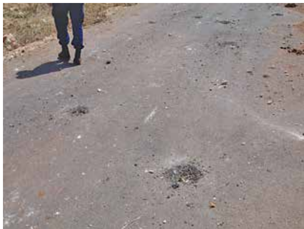
Image 3. BLU-63 impact patterns on asphalt, Yohmor, southern Lebanon, August 2006. Note how in asphalt the fragmentation may be tighter than seen on harder concrete surfaces. Photo courtesy of Steve Priestley.
