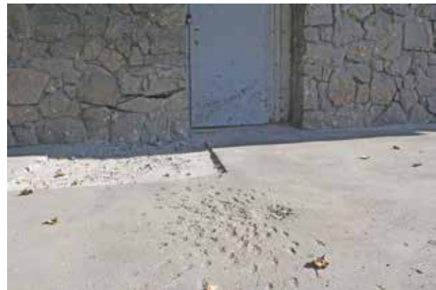
Image 5. A fragmentation pattern on a hard surface caused by 9N210 submunition impact near an ICRC office, Donetsk, October 2014. Photo courtesy of the Harriet Salem.
