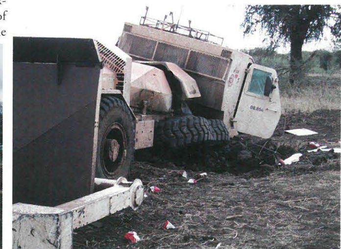
■ (Left to Right) The Finnish flail standing idle in Mozambique. A Hydrema flail in Ethiopia after it had detonated an AT mine that it had missed with its flail.
