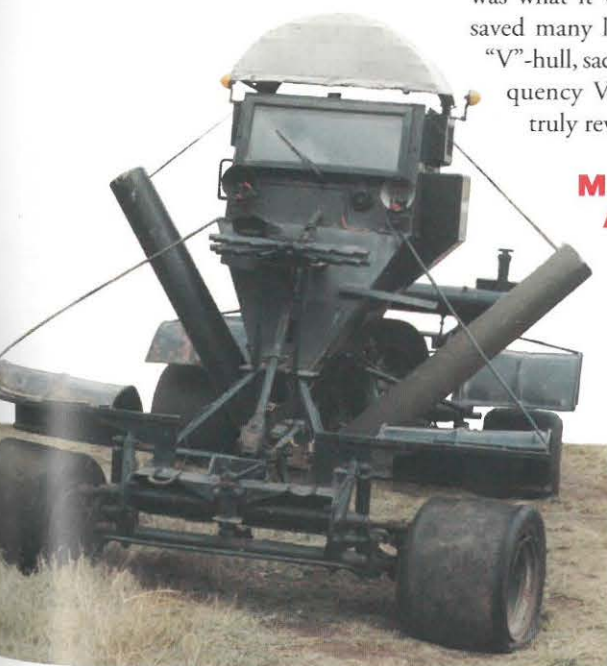
■ The Pookie: a single-seat mine-resistant mine-detection vehicle.
