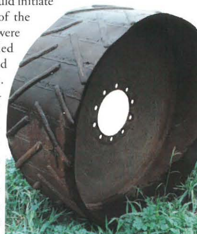
■ An example of a simple steel wheel—standing about 125cm (4 feet) high.
