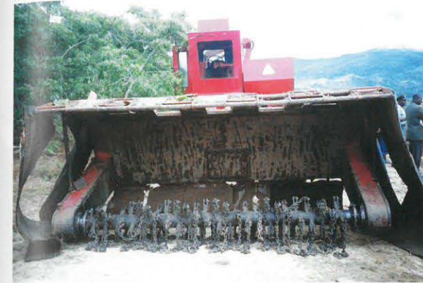
■ The MINETECH flail—a locally made monster that was far cheaper to make than any commercially available alternative.
