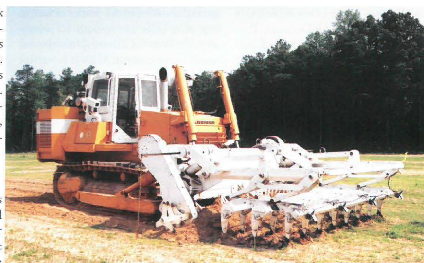
■ The Mine Clearing Cultivator is a vegetation clearance/ mine removal machine that is remotely controlled as well. This tool has been one of the R&D Program's most successful developments so far.
