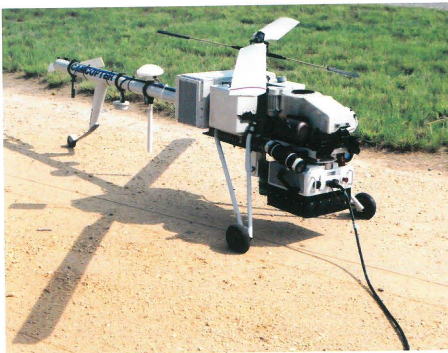
■ The remotely controlled Camcopter is a fully autonomous tool used to detect, identify, map and mark landmines while allowing the operator to be a safe distance from the minefield.
