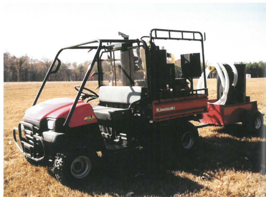
■ The AIR-SPADE is a safer way for deminers to excavate landmines proving itself especially useful in hard soil conditions. The airjet, which travels at a supersonic velocity, is powerful enough to break up tough soil, yet will not detonate mines.
