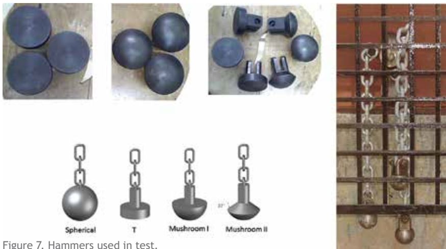
Figure 7. Hammers used in test. Figure courtesy of author.
