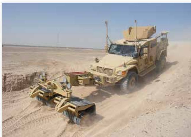
Figure 2. The Pearson mine roller. Photo courtesy of Pearson Engineering.
