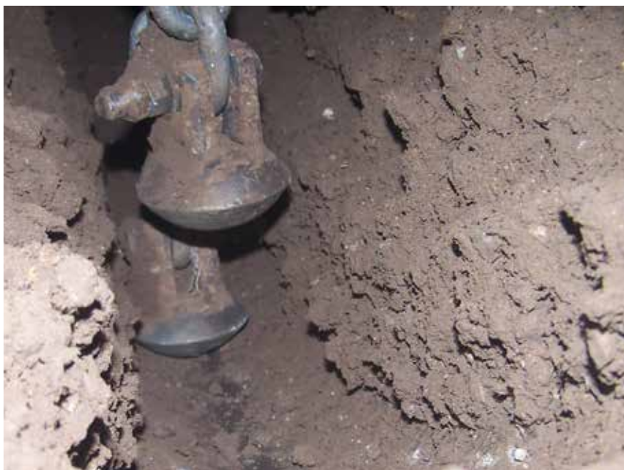
Figure 8. Soil container after test using Mushroom-I hammers in clayey silt. Figure courtesy of author.
