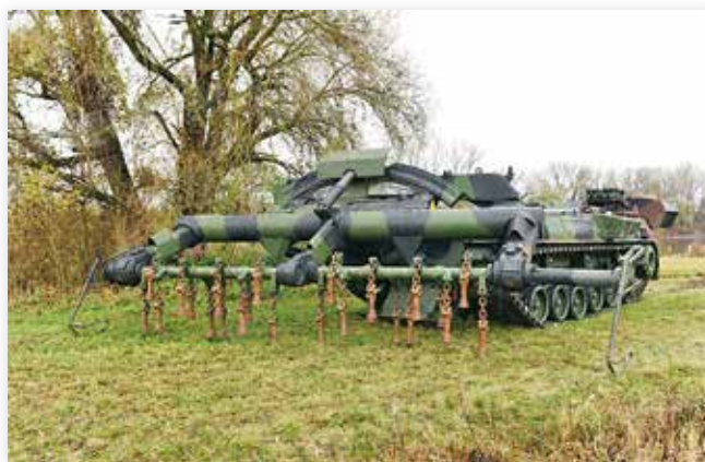
Figure 3. The Keiler mine flail. Photo courtesy of Rheinmetall.
