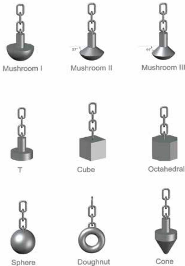
Figure 5. Types of hammers used in chain flails. Figure courtesy of author.
