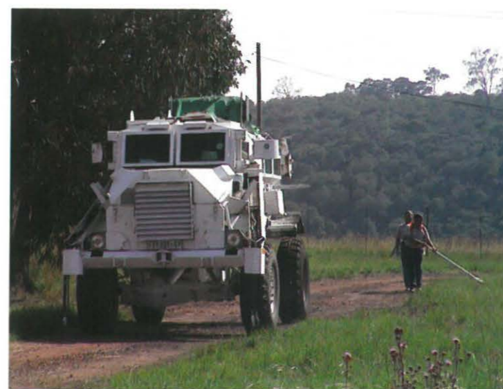
Casspir with an integral sampling system, used in the early days. The filter cartridges are seen hanging to the front of the vehicle. This is safe for the operator but offers limited control of the sampling zone. Portable sampling units are used behind, to ensure suction from vegetated areas.
