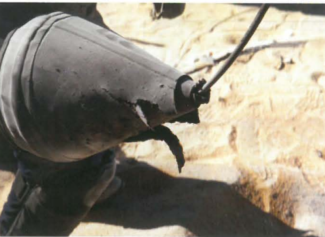
Figure 7: CHP-100 after having been exposed to the blast from a 200-g C4 mine at close range. While superficial damage has occurred, the overall integrity of the hand protector has remained intact. Note that the force of the blast severely bent the steel mine prodder.
