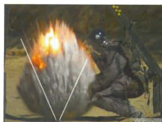
Figure 6: Photograph and schematic from live blast test demonstrating conical region of increased threat created by mine buried in soil. The ground and soil serve to confine and focus the blast effects. By remaining relatively low in orientation while still maximizing standoff distance, the exposure to this region can be reduced.
