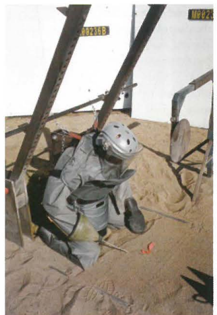
Figure 3: Test setup for full-scale blast testing. The mannequin, equipped with the LDE, LDH, OHP-100 and CHP-100, is placed in kneeling position with a nose-mine standoff of 80 cm. The mine position is marked by the orange flag.
