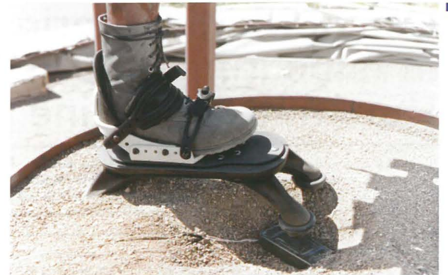
Figure 8a & 8b: Testing of Spider Boot on instrumented mechanical surrogate leg. First image shows a Spider Boot in place over a PMA-1 mine (200-g explosive). The second photograph was taken after the blast. The force of the blast has removed the front pods, by design, but the standard combat boot remained intact. The standoff distance introduced by the legs of the boots helps to dissipate the blast effects of the mine before they can interact with the foot of the user.
