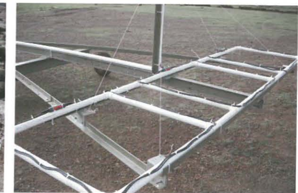
(Left to right) The main road leading from Berantu to Bushuka. Three UPEX detector coils mounted on PVC pipe to one of the earlier trailer systems. (Below) The computer workstation and control boxes for the UPEX detectors mounted inside the Samil 20 Mine Resistant Vehicle.
