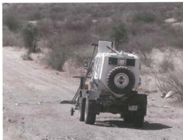
■ (Left to Right) A rear view of the front-mounted KIMS attached to the Samil 20. The side "wings" can be quickly folded up to work around trees and bushes. Figure 1: Sample Map.
