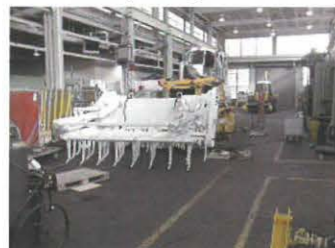
Mine Clearing Cultivator under construction in the NVESD prototyping facility.
