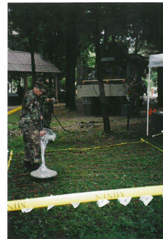
■ Figure 3. A U.S. Marine Corps Gunnery Sergeant operating the QR detection probe on the test area at Eagle Base, Tuzla, Bosnia. The probe, a laboratory prototype, is wrapped in plastic to protect it from the rain. A tether links the probe to a rack of electronics on the truck in the background.
