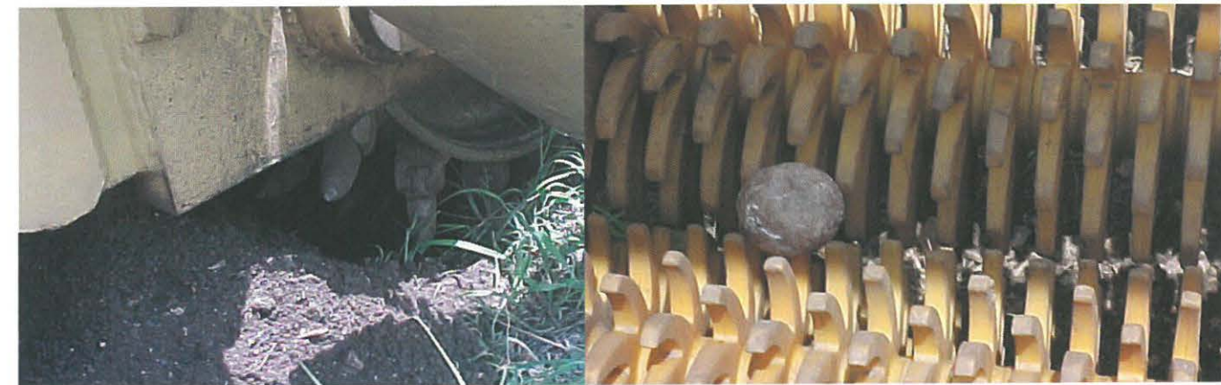
■ Grinding teeth and nylon finger rollers of the Minebuster. c/o Andy Smith
