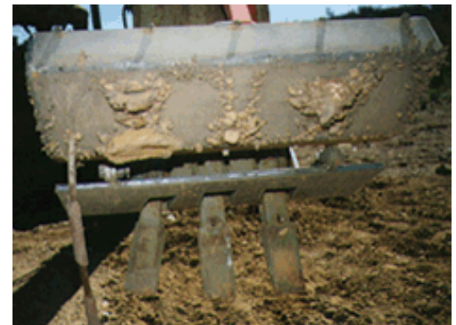
Figure 6: Fragments tend to collect along edges of slab magnets. Note long piece of steel pipe hanging from magnet at left-hand end.
