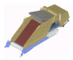
depth of 50cm, cleaning the soil of all manner of metal fragments, including ammunition, mines, and other unexploded ordnances (UXO). BIGAT acknowledges that the MiSa 1 is not appropriate for use on all minefield areas, but is encouraged by the results produced by the machine in tests thus far. The following article sets forth the detailed specifications of the MiSa 1, and examines the ways in which the machine may be used to aid mine clearance operations.
