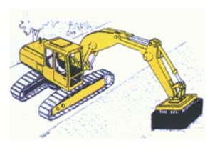
The picture to the left shows the demining equipment fitted to an excavator which has centre steering system. The excavator makes it possible to pass through areas with fluctuating passability.
