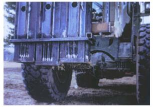
The spikes fitted to the Swedish Mine Fighter are closely fitted to each other which makes it possible to destroy or detonate even the smallest mine and it does not mater if the mine is on
