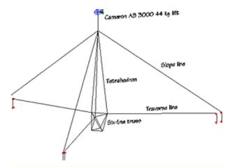
Figure 4. A perspective view of the control lines of the balloon system. Provided that all cables in the tetrahedron and six-line truss remain taut, they behave like a 'rigid' structure.
