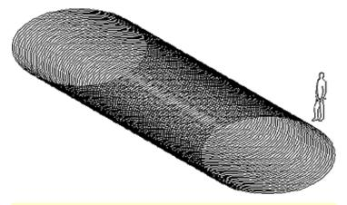
Figure 2. The overlapping circles of the Dervish track. Every point in the 5- metre wide path is covered twice by a load a little greater than that of a human foot.
