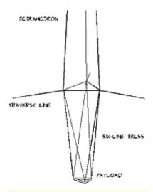
Figure 5. A less distorted view of the lines near the payload. The proportions of the six-line truss would be selected for a given mission to clear the highest obstacle and pass the narrowest gap.
