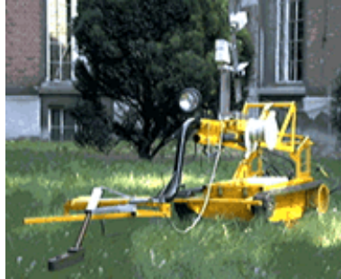
Fig. Tracked Hunter-Robot equipped with a metal detector
