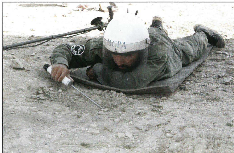
Self-monitoring prodder. Self-contained, no wires.
