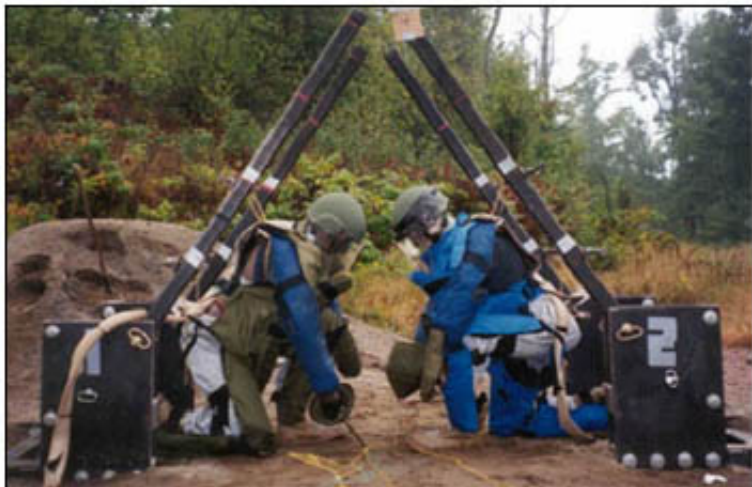
Typical setup for full-scale tests with mannequins. Mannequins donning HDE Demining Ensemble, HDH Helmets, and prototypical hand protector by MES.
