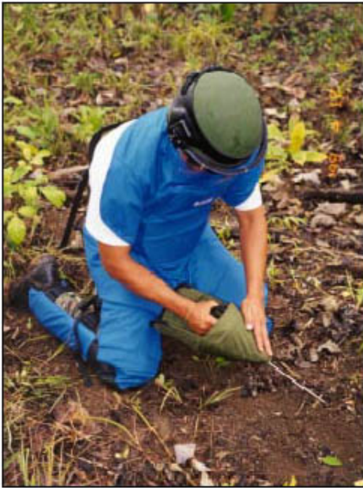
Deminer prodding for a mine in kneeling position while donning HDE Demining Ensemble, HDH-1 Helmet, and prototypical hand protector, by MES. Typical distance from sternum to end of prodder is 0.65-0.70m.
