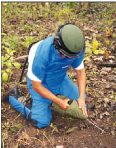
Figure 3: Deminer prodding for mine in kneeling position, donning HDE Demining Ensemble, HDH-1 Helmet and prototypical hand protector. Typical distance from sternum to end of prodder is 0.65–0.70m.
