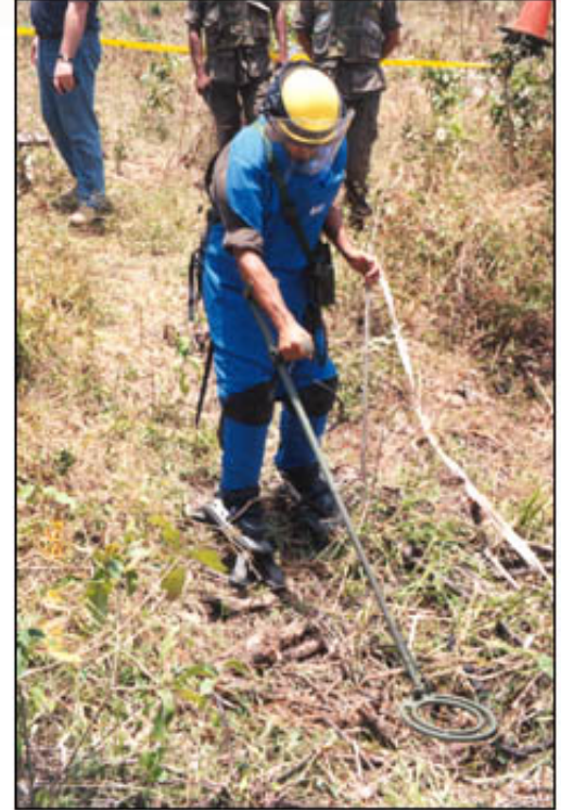
User trials of the Spider Boot with humanitarian demining suit by army personnel in Nicaragua.
