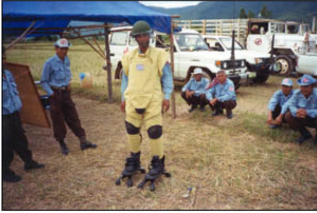
User trials of the Spider Boot with humanitarian demining suit by a deminer in Cambodia.
