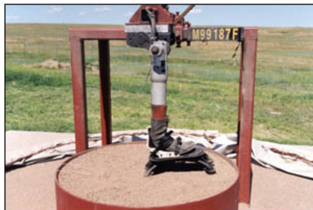
Instrumented mechanical surrogate leg used in DRES tests.
