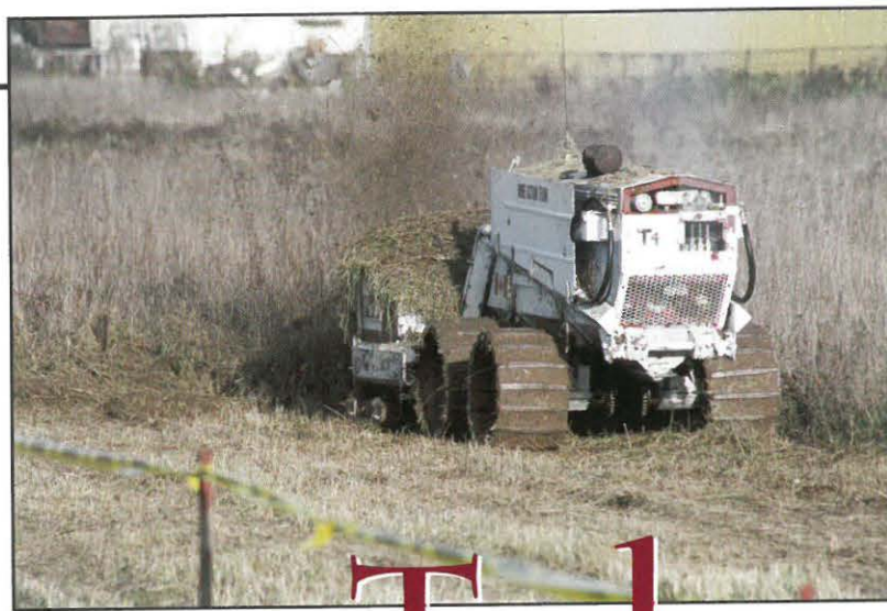
Tempest cutting vegetation in a live area in Bosnia Photo c/o Russell Gasser
