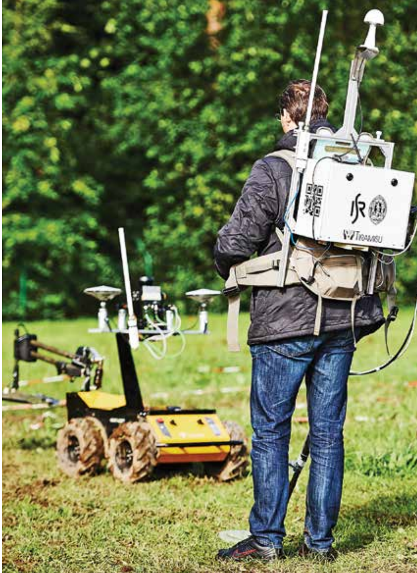
The arm of the remotely operated Semi-autonomous Demining Robot Husky-ISR/UC carries a triple coil metal detector, and the robot carries a sensor payload composed of video cameras, a 3D laser range finder, an inertial measuring unit and a GPS receiver.
