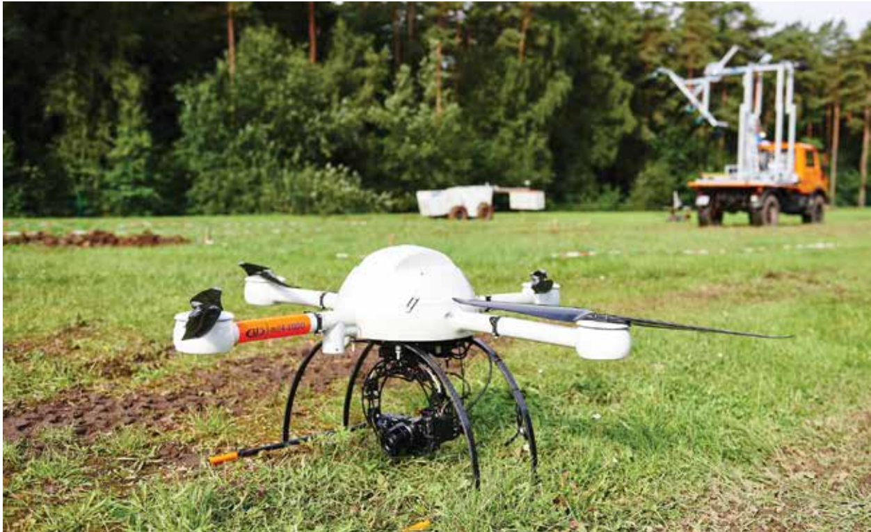
A few of the products demonstrated include the TIRAMISU drone, which provides 3D mapping capabilities, and the TIRAMISAR (in the background on the right), a side-looking imaging sensor with ground penetrating radar.
