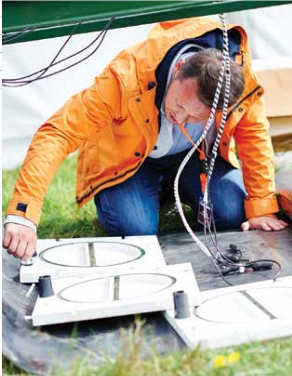
Haris Balta of the Belgian RMA prepares the Teodor V-Metal Detector D Array for a field demonstration.
