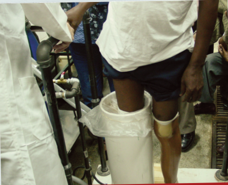
An amputee tests out the CIR Transtibial Prosthetic Casting System at the CIR training workshop at the Tanzania Training Center for Orthopedic Technologists.
