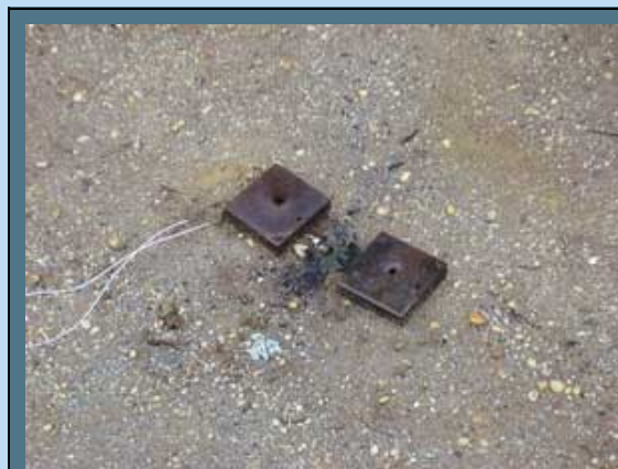
AP mine remains after deflagration.
