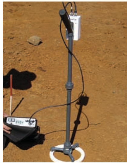
STEMD metal detectors tested according to the CWA 14747.
