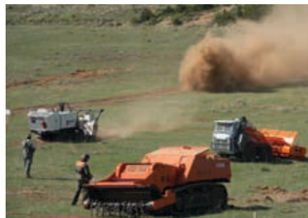
The Samson 300 is a manned machine that became totally engulfed in dust, making it nearly impossible for the operator to see where he was going. PHOTO BY LOIS CARTER FAY
