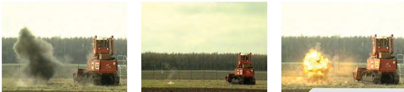
Figure 9: The operability of the MineWolf was not affected by fragment hits from the AP fragmentation mine DM 31.
