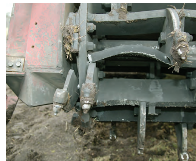
Figure 8: Damage after clearing a TM 57 AT mine.
