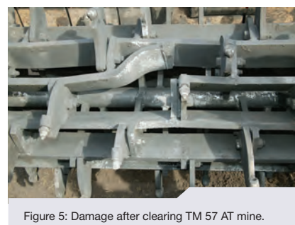
Figure 5: Damage after clearing TM 57 AT mine.
