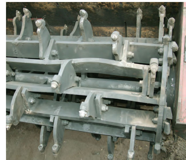
Figure 7: Damage after clearing a TM 62 P3 AT mine.
